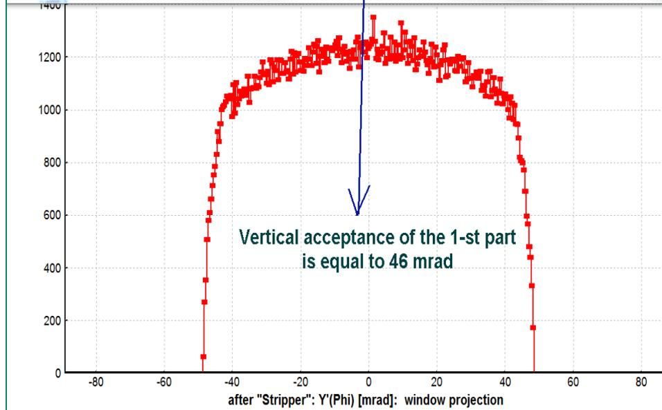
Angular acceptance  $X' = \pm 93$  mrad,  $Y' = \pm 46$  mrad (**Rectangle** shape) has been applied to the "Tuning" dipole.
