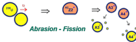
Figure 30: Schematic illustration of the abrasion-fission process.
