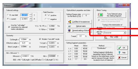
The new" solenoid block allows to select a block which map matrix will be used for tuning.
