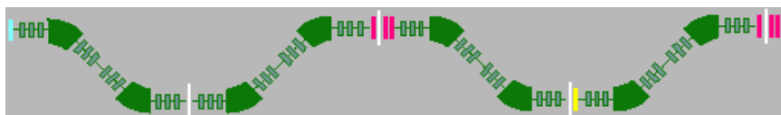
Fig.232. The spectrometer consisting of two A1900 fragment-separators built with the help of the “Append blocks from file” command.
