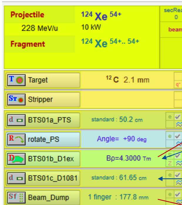
MC calculates the transmission "AFTER" the selected block, so do not use the Beam Dump block directly.
